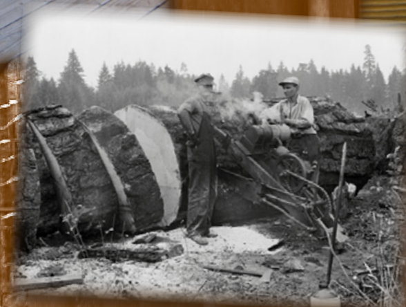
Once the drag saw was set in place – the operator merely stood back and watched it do the work. This allowed the crew to concentrate on splitting the rounds and feeding the fire box on the boiler.
