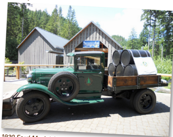
1930 Ford Model AA, 40 hp engine with 275 gallon water capacity. Trucks like this one were among the first used by wildland firefighting crews in Oregon. This replica pumper truck restoration was completed in 2011 by the Southwest Oregon District to commemorate the Department's 100 th anniversary.
